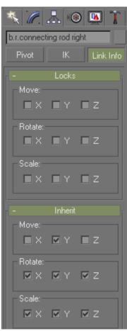
Link 'b.r.piston right' to b.r.connecting rod right'. In the 'Hierachy' tab set the 'Inherit' and 'Move' check boxes for 'b.r.piston right' as shown.
