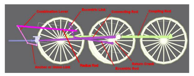
By the way, when the loco is in forward gear the joint between the Radius Rod and the Eccentric Link is below the pivot point of the Eccentric Link, and when in reverse gear above it. In real models (and most virtual ones!) a common dodge is to model the gear in 'neutral', i.e. the Radius Rod pivot is coincident with the Eccentric Link pivot. This means that the Radius Rod doesn't move which is a pity.
