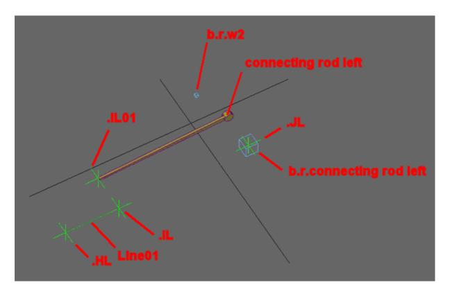
It's not as bad as it sounds actually. Create dummy called ,b.r.connecting rod left' in top view and align it in X,Y and Z to point ,.JL'. Create a line ,Line01' between ,.HL' and ,.IL'
