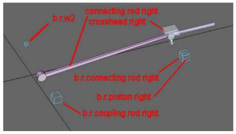
The first step is to link 'b.r.coupling rod right' to 'b.r.w2'. Hide everything you are not working on and use the 'Link' tool to create links between the objects by dragging. Create 'b.r.coupling rod right' in top view and centred on the crank pin of the driving wheel.
