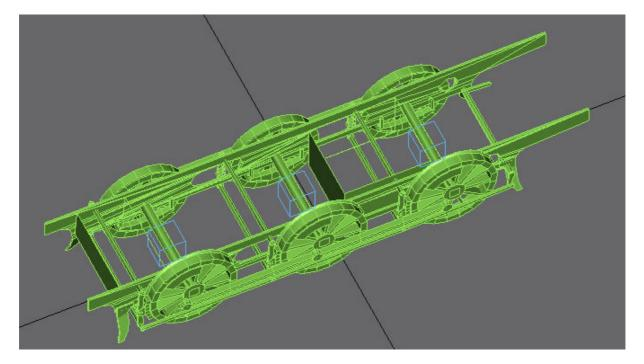
We'll need to sort out the rest of the bogey mesh now, as the parts that should belong to each wheel set need to be detached from the main mesh and reattached to the appropriate wheel rim. Obviously if making your own bogey you will have planned ahead a bit better and not attached everything together in the first place...
