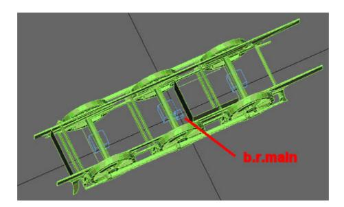
These days I would leave it there to make things easier, but the attachment point in the loco body is set at axle height so I need to align the Z coordinate of the dummy 'b.r.main' to one of the wheels.
