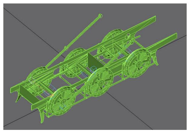
Never mind, this is easily fixed. Select the dummy 'b.r.rod\_left' and select the 'Hierarchy' tab and 'Link Info' and uncheck the 'Inherit -> Rotate X' box. This prevents the dummy from following the X rotation of the wheel, which is exactly what we need to keep the coupling rods level as the wheel rotates.
