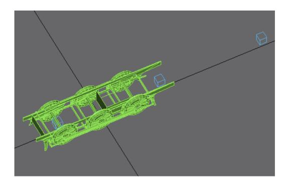
Rename the two new dummies 'b.r.wheel2' and 'b.r.wheel3'. Align the dummies to the wheel rims 'rim2' and rim3' in the same way that we did for the first dummy so that all of the dummies are centred on the respective wheels.
