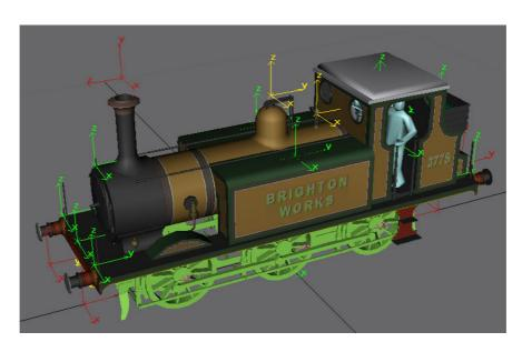
The planes can be mirrored over to the other side and the UVW coordinates can also be mirrored to avoid the texture being mirrored as well.
