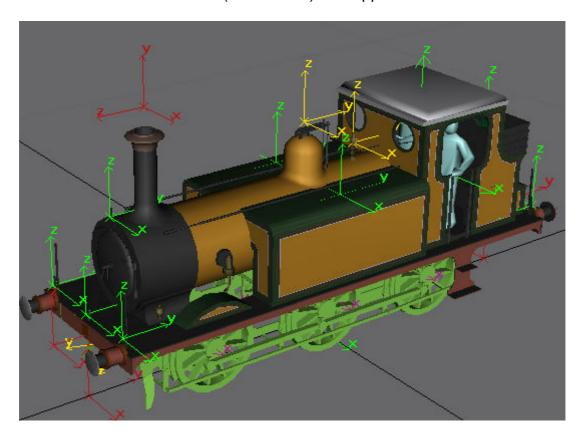
Before we end this part I'd like to point out that a common mistake when skinning is to use colours that are too strong. In this case the bottommost layer in the PSP file is filled with 51,51,51 dark grey. If we hide the mapping layer and reduce the opacity of the yellow body colour layer we can tone down the overall brightness of the skin to create a more natural look.
