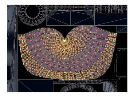
Scale the mapping down by pressing S with the cursor over the UV/Image Editor window (I suggest to 80%) and detach the offending object from the body mesh. The object needs to be detached as there appears to be no option to bake just selected faces. Deselect the 'Clear' button in the 'Bake' panel and change the 'Margin' setting to about 8.
