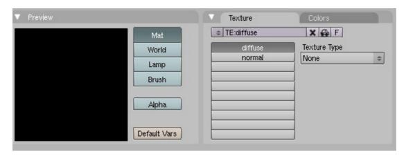
Here we can see the two channels that we have defined, but we actual textures have still not been assigned. The 'Texture Type' for both channels needs to be changed to 'Image' (default is 'None').
