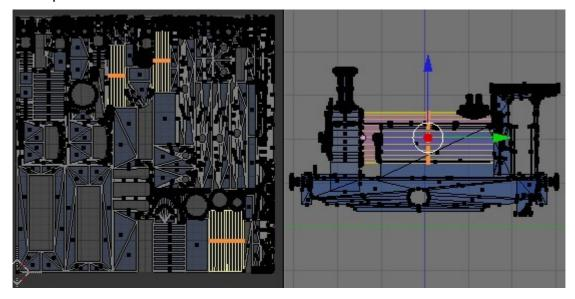
To optimise this switch the 3D view to Top Ortho (press 7 and then 5 if needed to get an Ortho view) then press U with the mouse cursor over the 3D window and choose 'Cylinder from View'.
