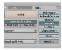
Hit 'Bake' to generate the normal map. As you can see the rivets have been projected on to the footplate. To make use of the normal map it is necessary to create a material that uses it and apply it to the mesh of course.
