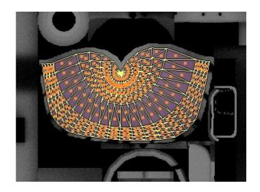
The dome can now be joined back to the body mesh and the process repeated for any other problematic areas.
