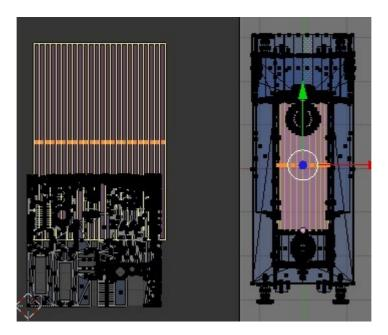
The boiler has now been mapped to a single rectangular area. To make the new mapping for the boiler the right size select all the faces and hit CTRL-A with the cursor in the 'UV/Image Editor' window. This rescales the selected UV maps depending on their relative areas in the 3D window.
