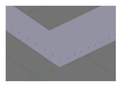
To normal map these faces we need to change a couple of things in the 'Bake' panel. Firstly deselect the 'Clear' button – this will overlay the new mapping on the current image without clearing it first. This enables us to create the normal mapping in easy stages. Secondly select 'Selected to Active'. This takes the selected object (the rivets) and projects it on to the active object (the footplate). Remember that the last object selected is always the active one.
