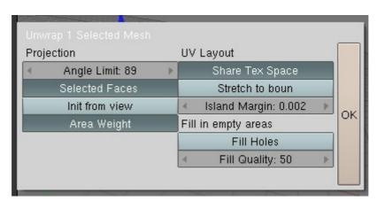
A few remarks on the settings – setting the Angle Limit as high as it will go (89) tends to create fewer islands. The 'Island Margin' separates the islands slightly which I find helps when texturing. 'Stretch to boun' (sic) should be deselected to avoid distorting the mapping.
