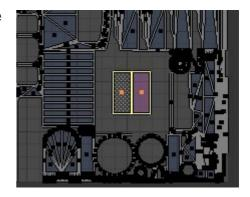
The islands can be selected, moved around (key G) rotated (key R) and rescaled (key S) just like mesh objects to make better use of the space. To select an island we can select a face and press CTRL-L, or use the new 'Island Select' mode introduced in version 2.48 (highlighted in the following picture, right click to select a whole island).
