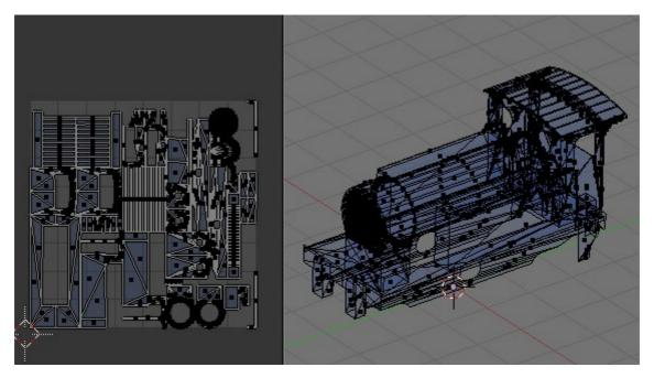
The model with a little manual optimising of the mapping is available <u>here</u>. **Note that the mapped faces are on layer 2, the rest of the mesh on layer 1**.All that remains is to map the rest of the mesh and arrange it on the UV map...
