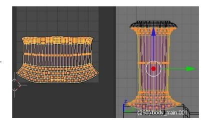
Move the three maps somewhere in the dark grey area of the UV/Image Editor window so that they are not overlapping (to make selecting them again easier) and join the chimney back together again, welding the vertices.
