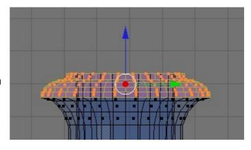
With the faces of the cap selected and the mouse cursor over the 3D window press U and choose 'Unwrap' from the menu. The cap now looks as though it has been flattened in the UV/Image Editor window as shown here.
