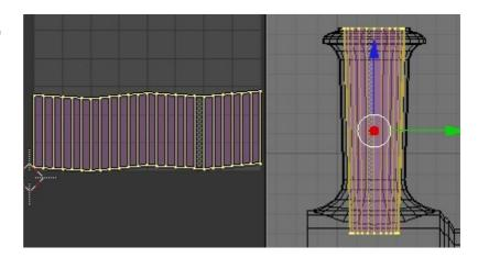
The wavy edges can be tidied up by selecting the vertices in the UV/Image Editor window and pressing W and choosing 'Align Y' from the menu. Make sure that the two highlighted icons are selected!
