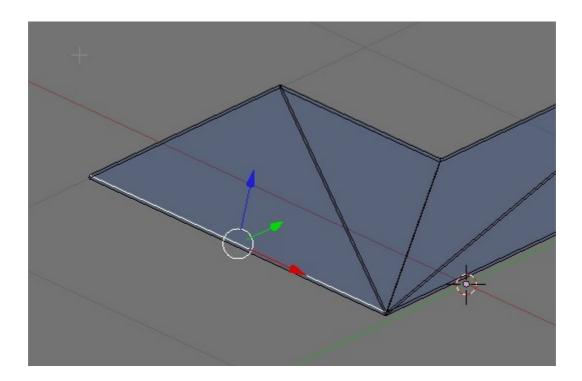
Press E (to extrude) and then Z (to constrain movement to the Z axis only). It's best to do this in the side view so that you can see how far to extrude by referencing the plan. So, mouse cursor over the Right Ortho view and press CTRL up arrow.
