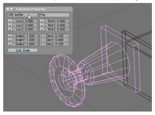
You can rename the buffer object at this stage using the 'Transform Properties' dialogue box (press N if it is not open already). Clean up the mesh by going into Edit Mode, select all the vertices, press W and choose 'Remove Doubles'. This will remove the duplicate
