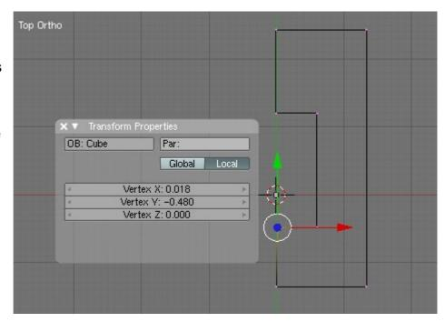
To create a mesh from this shape select all the vertices and press SHIFT-F:
