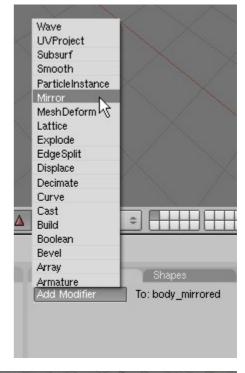
Done. Now that the mirror modifier has been applied any modification to the left hand side of the mesh will be automatically applied to the right hand side.
