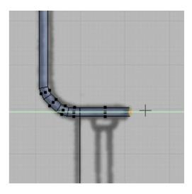
On the other side I've shortened the beading up to the start of the radius for the handrail extension and have positioned the 3D cursor to the approximate centre of the radius.
