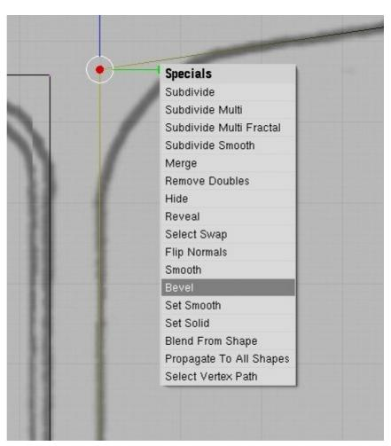
Drag the vertex with the left mouse button to create the bevel. Bevel the two new vertices again to finish the fillet.
