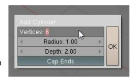
the value of 'Vertices', the default is 32 which is higher than you'll need even for a boiler. Watch out how many segments the final cylinder will have, they can cause the polygon count to increase rapidly.
