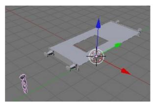
All that remains to do is to move the coupler (the snap tools are handy here) to the front of the buffer beam and to duplicate and rotate it for the rear beam.
