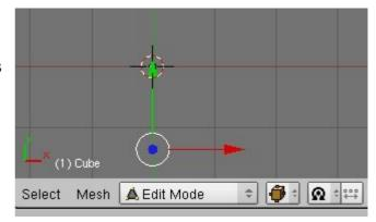
Now we'll extrude the vertex to create the rest of the shape with by hitting E and then X to extrude to the right (direction +X):
