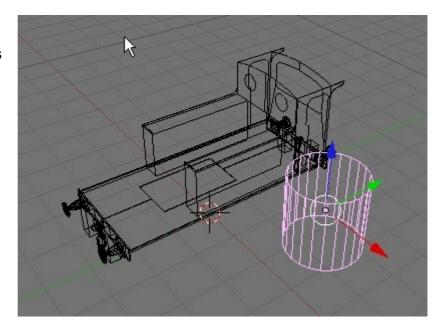
And now rotated and scaled to match the scale drawings... The smokebox has been created by extruding and scaling the front end of the boiler, this is easier if the boiler is a full 360°.
