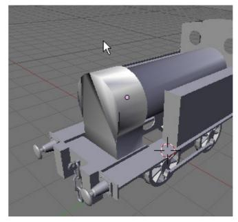
Go into 'Edit Mode' on the boiler object and select one of the faces on the smokebox front, then press ALT-CTRL-SHIFT-F. All the adjacent faces on the smokebox front will be selected, but not the curved sides.
