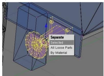
Break the buffer out of the mesh, rename it in the 'Transform Properties' dialogue box and delete the mirror modifier on the object.
