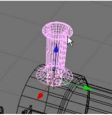
Finally in the 3D view and in shaded mode the edges of the base of the chimney must be moved in Z so that they just touch the smokebox. In the side view adjust the other vertices to make a smooth base for the chimney.
