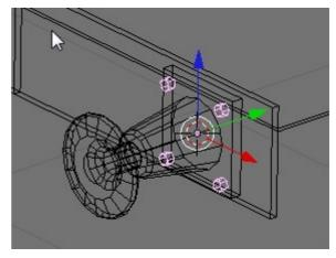
Joining the bolt heads to the main mesh will mirror them over to the other side automatically.
