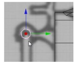
In this case the handrail is centred on the boiler, so set the 3D cursor to the boiler centreline and using 'Spin' create the first part of the handrail in the front view. You'll have to guess what angle is needed, in this case it was 45°, but if you get it wrong just hit CTRL-Z and try again.
