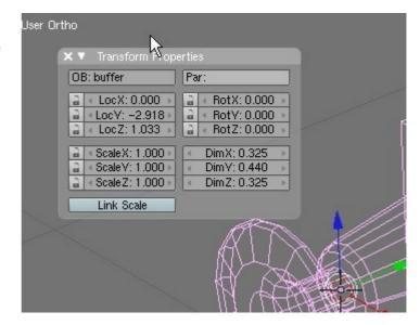
For UK locos the buffers were almost always at 5'8" (1.727m) centres and at a height of 3'5" (1.041m) above rail level. The Z height of the buffer in this case is only 9mm too low which is near enough, and the X coordinate is 0. This needs to be changed to 1.727/2 = 0.864. Type this into the 'LocX:' field and hit ENTER. The buffer will jump to the new X coordinate.
