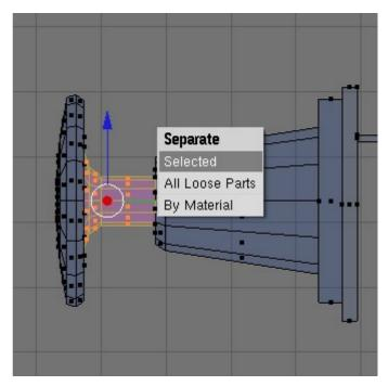
When you split an object that has a mirror modifier applied the modifier is also applied to the mesh that you split out. Joining two meshes with a mirror modifier seems to confuse Blender, so it is best to delete the modifier on the mesh that you have separated.
