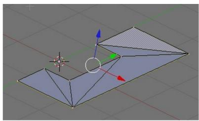
Switch to the Right Ortho view (mouse cursor over it, CTRL up arrow to maximise it) and adjust the footplate to match your background image. To do this you need to use the B key to make a box selection, A to clear selections and the GY and GZ key presses to move the vertices to the correct positions. Once you've sorted out the side view do the same for the front view to get things the correct width.
