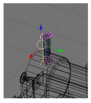
Switch to 'Object Mode' and apply a mirror modifier in X and Y to complete the chimney, but don't forget to move the pivot point to the 3D cursor first as the mirror needs to be about the centre of the chimney.
