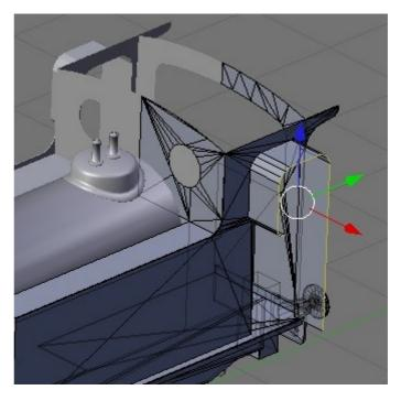
Select all the faces of the bead/frame and apply the 'Solidify Selection script with a suitable value to add thickness.
