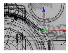
Switching to the top view the handrail was completed with an extrusion in X, a 90° spin with 3 segments around a new position for the 3D cursor and an extrusion in the Y direction.
