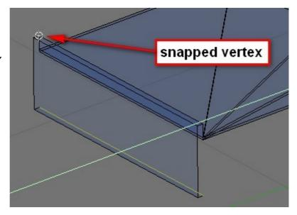
Switch now to face select mode and select the faces belonging to the buffer beam using right click and SHIFT right click. When in face select mode each face has a small dot at its middle point making it easier to select. The .faces turn pink when they are selected
