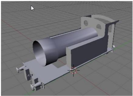
The vertical sides of the smokebox were made by deleting the 8 faces at the bottom of the circular smokebox and extruding the free horizontal edges downwards. The new faces were then detached with P and moved and resized to match the scale drawing. The area between the vertical faces and the circular part of the smokebox was filled by extruding a few faces. The front face of the smokebox was made by selecting the vertical free edges and pressing SHIFT-F.
